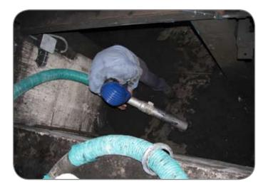
Foundry: Classic work in the foundry. Cleaning of pits with difficult practicability from fine heavy foundry sand. Operators that work normally with shovel and bucket are able to suck 1000lt of material in 12 minutes with Nilfisk CFM HPV Compact container of 37kW. Discharge easy by pull out the container and discharge thru bottom unload where it is useful for the customer. The material can also be recovered and brought back in production process.
