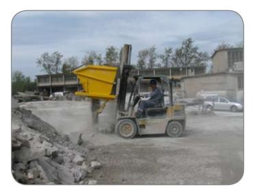
Cement Company uses the Nilfisk CFM HPV Compact as flexible to use clearing tool mainly in the Milling area to remove the Big quantities of Klinker dust with hoses up to 50mt.
