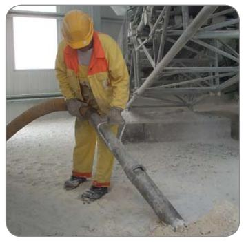
Nilfisk CFM HPV centralized vacuum system connecting 2 production towers with the pipeline for removing the dust and debris created during the milling and working process inside the production towers. All the removed material is discharged automatically on the belt that brings the material back in the production. Cleaning, maintenance of the plant removing the abrasive dust and stones and recovering of Material in one system.
