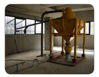
Pipeline in the Incinerator connected to the Nilfisk CFM HPV Cyclone separator to suck heavy or big size material, mounted on a higher level discharge the material continuously in the Big Bag or Customer container on the level below.
