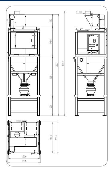
Decontamination: use of the Nilfisk CFM Compact on hopper to suck big quantities of contaminated Debris during the demolition of an Industrial building. The material sucked is contaminated by Heavy metals and asbestos. For this reason the machine was equipped with M – class filter Bags and efficient Downstream Absolute Filter H14 class.
