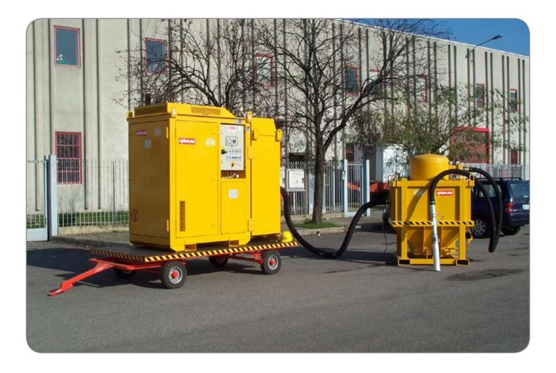
Cleaning contractor ordered N°4 Nilfisk CFM Multivac Models on trailer connected to 1.300lt. separators with bottom discharge for the use in a wide chemical area.
