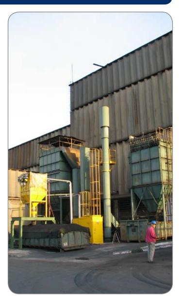
Nilfisk HPV Multivac electric 55kW, connected to the HPV separator as stationary Filter system Bag house, with continuous Filter cleaning by compressed air purge system. The Separator is connected to a reinforced stainless steel pipeline that pass through the complete areas of foundry sand recycling to collect the foundry sand that has to be eliminated from the production process. The Hopper below the bag house discharges continuously in the customer container.
