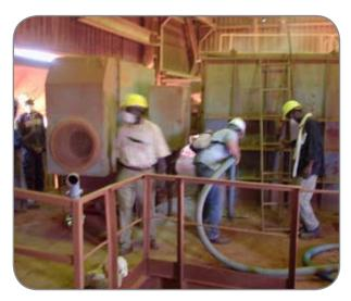
Bauxite Mining Industry needs to clean in the milling, cooking and silo area. Abrasive dust and debris need to be removed from moving parts and Conveying belts. Cleaning and maintenance. The company decided to invest in machine as people are not able to provide requested high grade of cleanness and fast removing of material that avoid production stops and machine damage.
