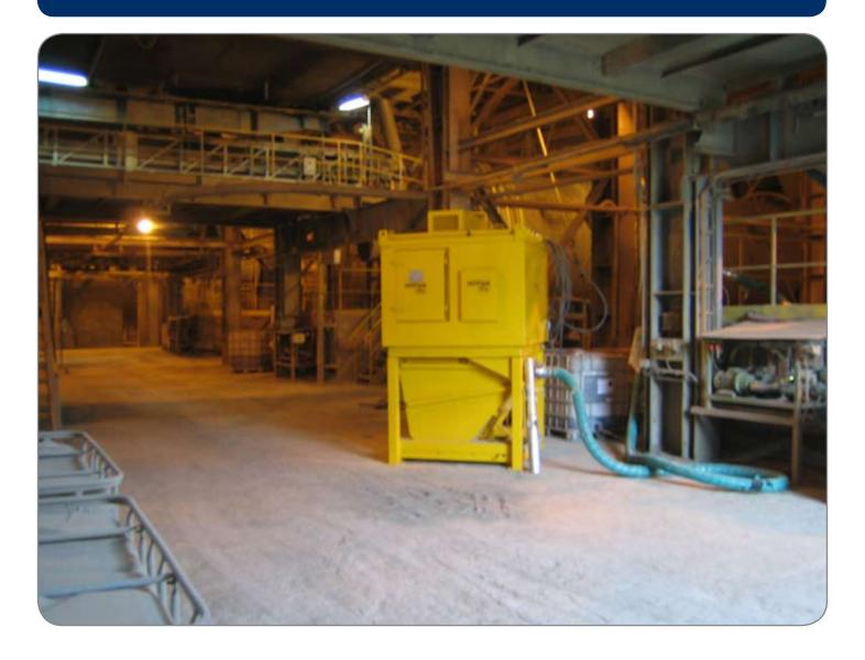
General cleaning in cement company: standard Nilfisk CFM HPV mod. Compact on Container used for the flexible, transportable use to clean and remove big Quantity of Bulk material.
